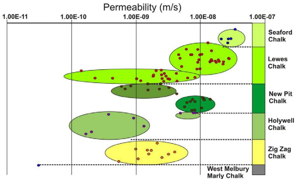
*Figure 2 - Distribution of permeability tested on core samples, in the laboratory at the University of Brighton, in relation to the lithostratigraphy of the Chalk in the FLOOD 1 catchments.*
