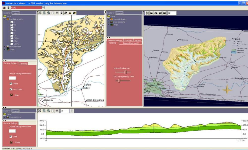
Figure 4 - 3D geological model of the Hallue catchment showing the ground profile and geological structure. Constructed using GSI3D.
